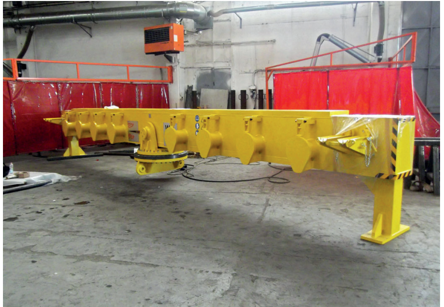
BILANCINO GIREVOLE / TURNING LIFTING BEAM PORTATA / CAPACITY 52.000 Kg
