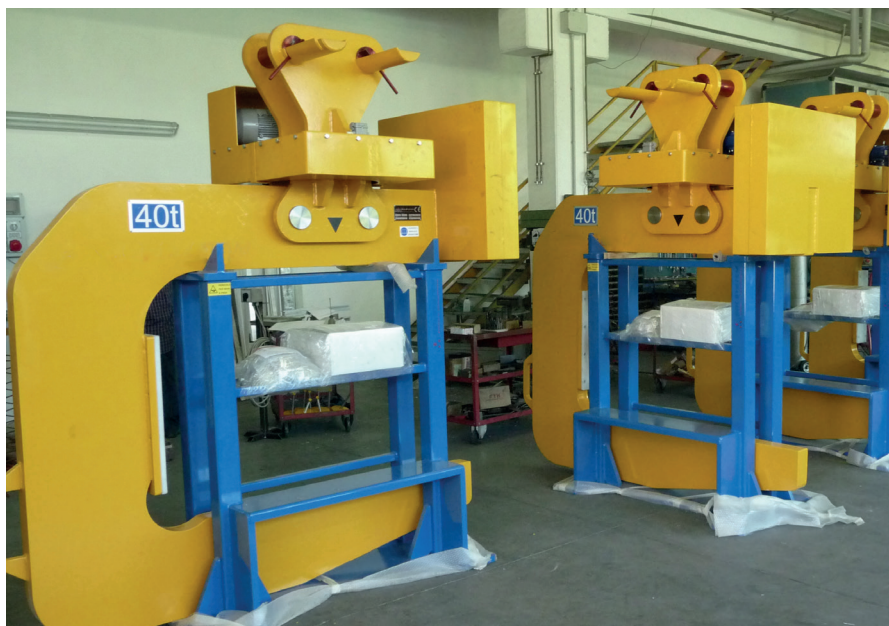
GANCIO A "C" PER COILS / COILS C-HOOK PORTATA / CAPACITY 40.000 Kg
